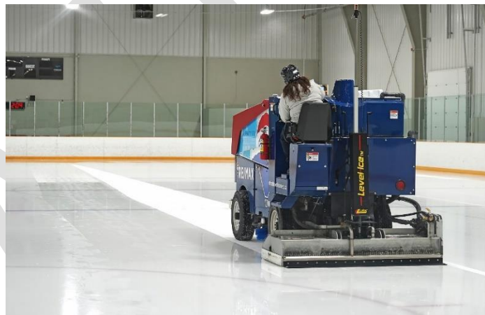
Figure 5 Electric ice resurfacer in use
